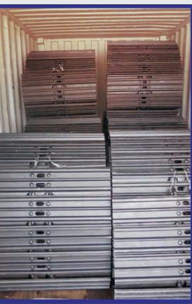
BERCH track chains are manufactured with 35MnB steel by forging. The hardness is HRC 52-57 and the deepness is 6-8mm after medium frequency quenching. We are developing lubricated track chains for bulldozers such as D65, D85, D155, D6D, D7G, D8K etc. Track Shoes are also available to supply.
