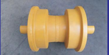
BERCH track rollers are manufactured with 50Mn steel by forging. The hardness is HRC 52-57 and the deepness is 5-8mm after medium frequency quenching. We use best quality floating seals, O-rings and Bi-metallic bearings to make sure a long wear life and impact resistance.
