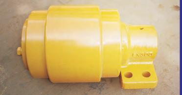
BERCH carrier rollers are produced with 50Mn steel by forging. The hardness is HRC 50-55 and the deepness is 5-7mm after medium frequency quenching. We use the same floating seals, O-rings and Bi-metallic bearings as track rollers.
