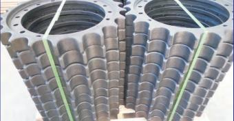
BERCH sprockets are manufactured with 40Mn steel by casting. The hardness is HRC 47-52 and the deepness is 11-13mm at the top and 4-6mm at the bottom after medium frequency quenching. We are developing forging sprockets to get better quality and appearance.
