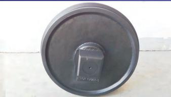
BERCH idlers are manufactured with 40Mn steel by casting. The hardness is HRC 52-57 and the deepness is 5-8mm after medium frequency quenching. We are developing forging idlers to get better quality and appearance.
